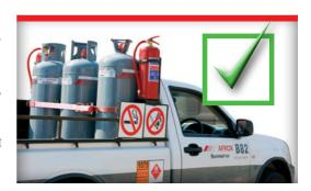
As LPG is heavier than air, any accidental release of gas will sink to the lowest point. Therefore, cylinders should always be **kept away from**:
